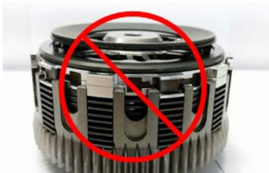
Incorrect – The Belleville spring is upside down.
