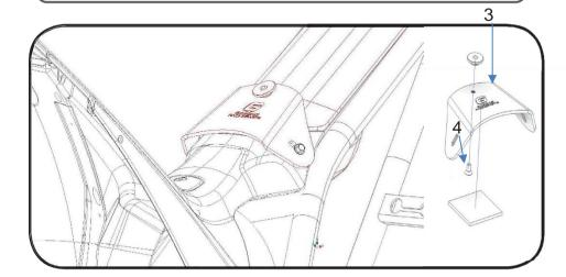
MAKE SURE PART N°3 IS THREADED TOGETHER WITH THE SUPPORT AND SCREW N°4. PLACE THE PROTECTIVE FOAM AND SCREW TO THE SEAT BASE WITH SCREWS N°6
