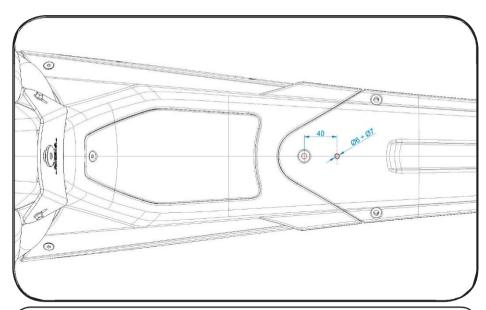
DRILL THE REAR FENDER AT 40 WITH A DRILL AND A 6mm DIAMETER BIT AS INDICATED IN THE ABOVE SKETCH. IT IS VERY IMPORTANT THAT THE HOLE DOES NOT REMAIN INSIDE THE FILTER BOX
