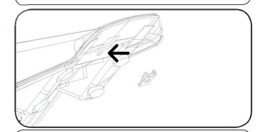
PUT THE CLAP ON THE LOWER PART OF THE SEAT. PLACE THE SEAT FROM THE FRONT PART AND FINALLY SCREW THE ENTIRE PACKAGE WITH SCREW
