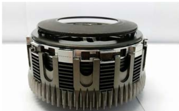
Correct – The Belleville spring sits flat against the slider ring.
