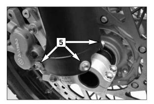
Attach the fork protectors to the fork leg axle passages with the six original M6x12.5 screws [5]. You will need to bend the right fork protector.
