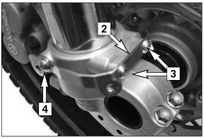
Mount the two adapter rings using two spacer plates [2], two M6x16 oval head screws [3] and one M6x12 oval head screw [4] for each ring.
