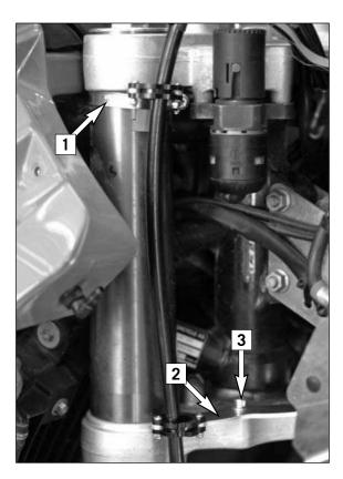
Use the pipe clamp [1] to mount the upper guide (tab facing down) and the retaining bracket [2] to mount the lower guide with two M6x12 oval head screws [3] on the brake line. Place the cable support sleeves in the guides and screw on.
