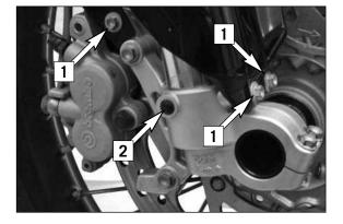
Remove the original fender. It is attached to the two fork leg axle passages with six screws [1]. An extra thread [2] will be required to attach each of the fork protectors and must be exposed.
