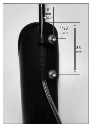
To mount to the fork protector, drill 2 holes in the holder (15mm from the center to the right and 30 mm and 85mm down from the upper edge) with a diameter of 6mm. Screw the clamps on the steel-wrapped brake line to the fork protector using the M6x20 HH collar screws and self-locking nuts.
