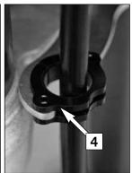
Slightly bend up the plastic brake line guides and slide over the brake-line. Press the plastic brake line guides [4] into the retaining brackets. Screw to each retaining bracket with  $2 \times M3$  oval head screws and 2 nuts.
