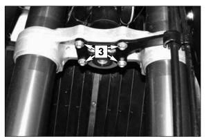
Also dismount the guide for the remaining original brake line by removing the 4 screws [3] from the lower triple clamp.
