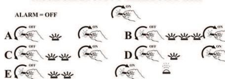
B) Within 3" return the ignition key to the OFF position and wait for the LED to start flashing in order to confirm the second digit; confirm the digit and repeat steps C-D and E for the remaining digits.
