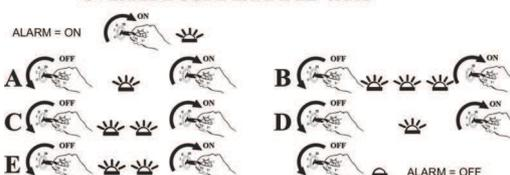
CAUTION: THE NUMBER OF FLASHES MUST MATCH THE FIRST DIGIT IN THE CODE (E.G. IF THE FIRST DIGIT IS 1, TURN THE KEY TO THE ON POSITION WHEN THE LED HAS FLASHED ONCE)
