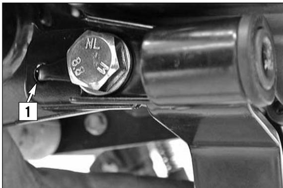
Remove the rear engine support bolt and the holder for the manifold.
