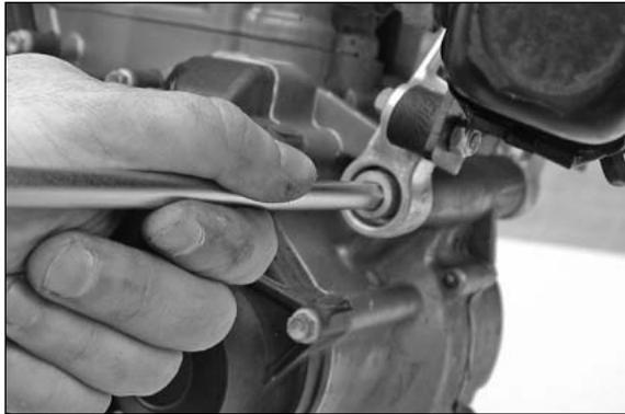
Remove the fuel tank, lambda probe, heat shield plates of the main silencers and manifold.
