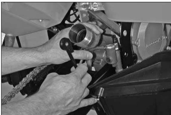
Loosen the heel protector fixture.
