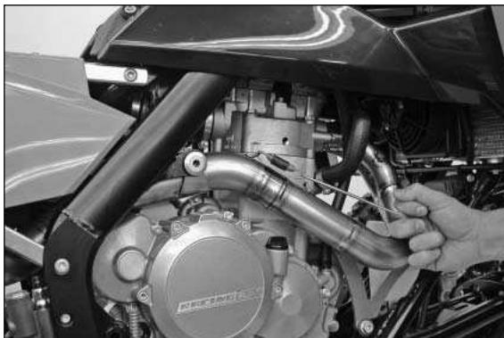
Connect the Akrapovic header fitting and header connector.
