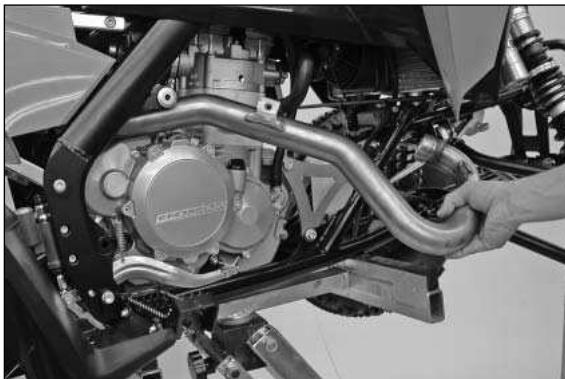
Remove the mounting screw on the standard header and remove the exhaust spring from the exhaust flange.
