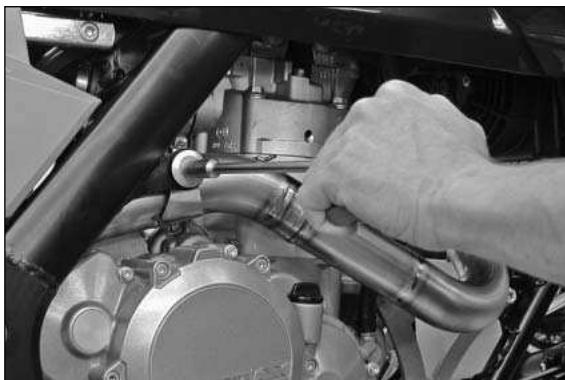
Do not tighten the M8x30 screw until the header pipes are mounted stress-free.
